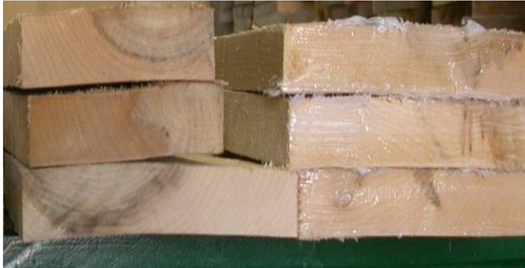
Figure 18 Boards protected with paraffin (left) and silicon (right) coatings against checking
