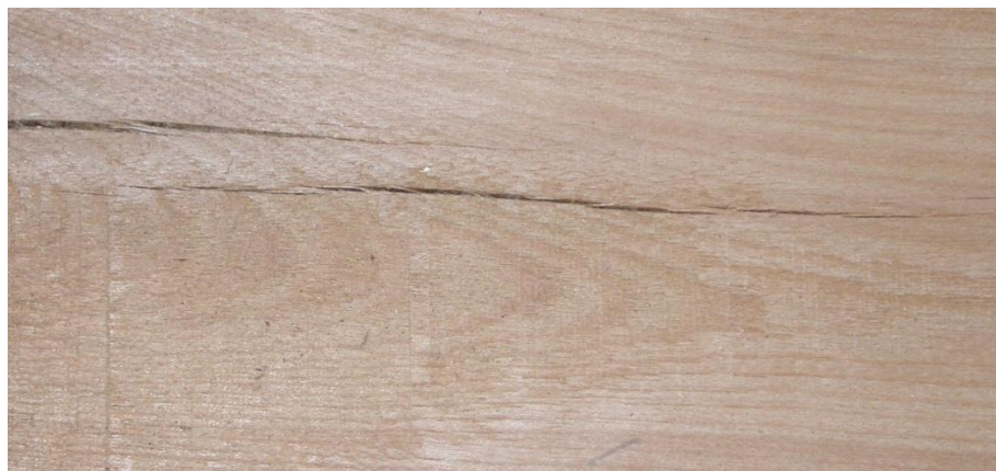
Figure 4 Surface checks in the middle of a board
