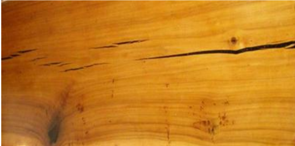
Figure 9 Splits formed on a finished board
