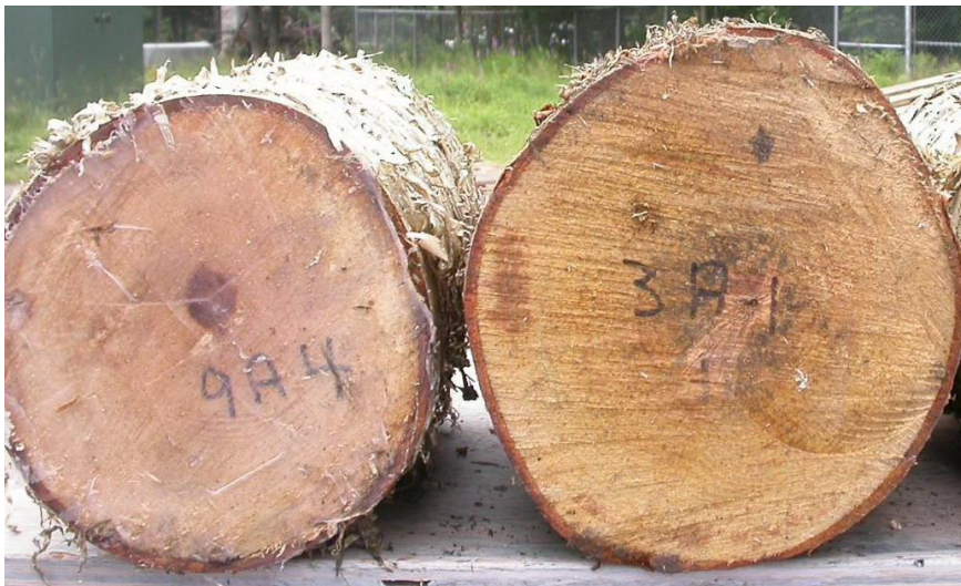
Figure 17 Logs protected with silicon (left) and paraffin (right) coatings against checking
