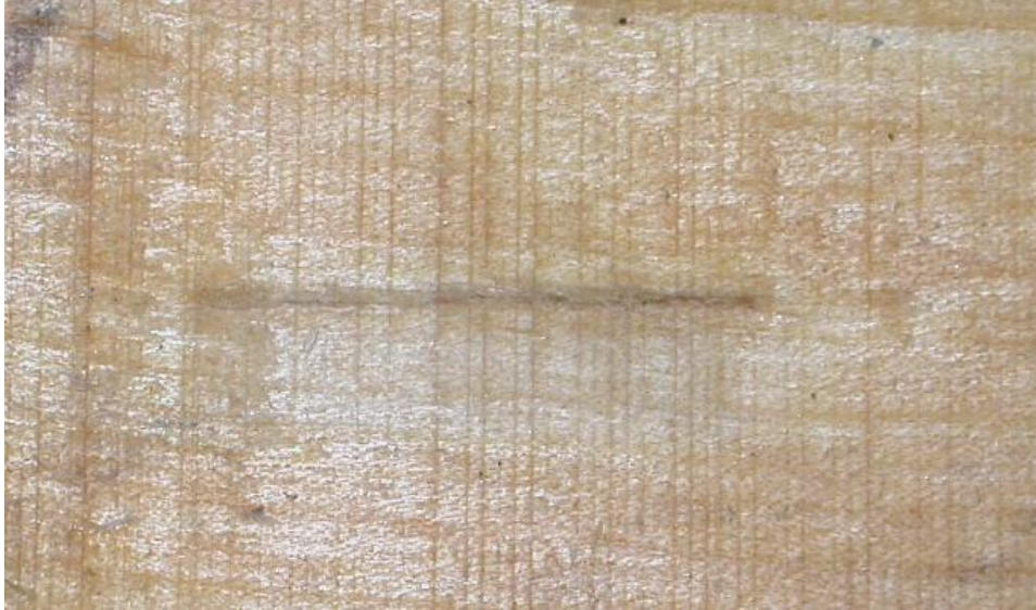
Figure 13 Harvester damage on a roughly-sawn sugar maple board
