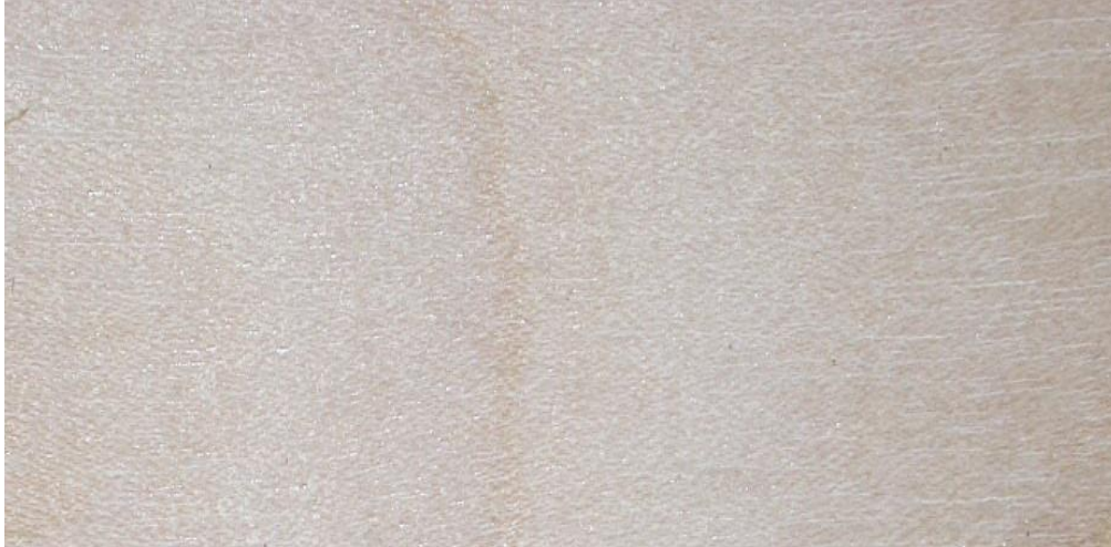
Figure 19 A wood component protected with a wax emulsion against checking
