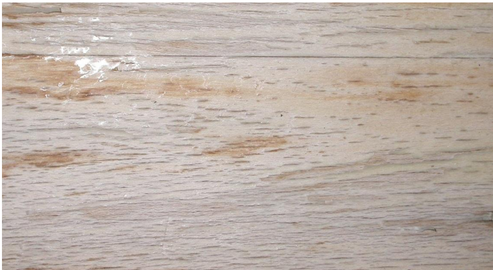
Figure 23 Checking on wood product with a peeled clear film-forming coating
