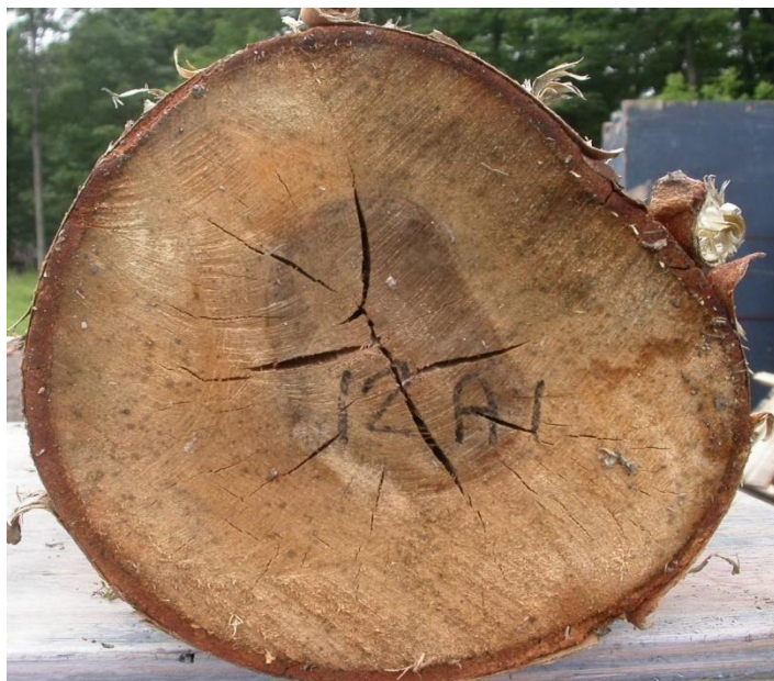
Figure 1 End checks occurred on a bark protected log
