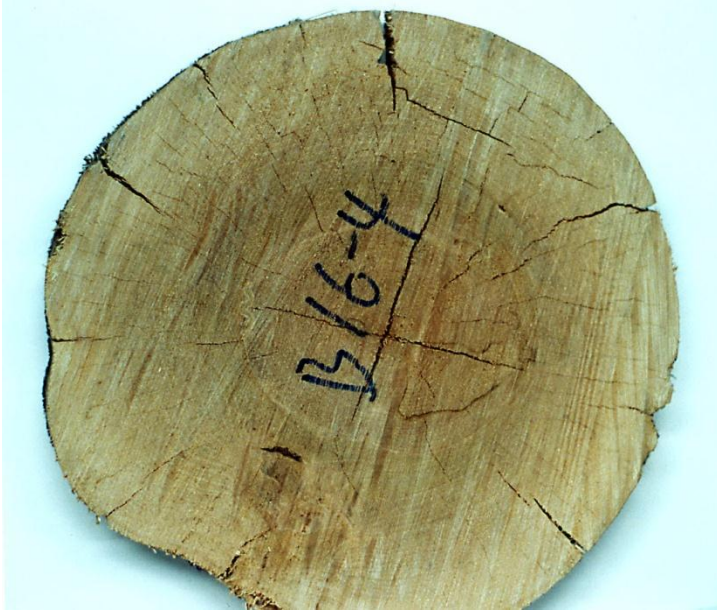
Figure 2 End checks occurred on a debarked log
