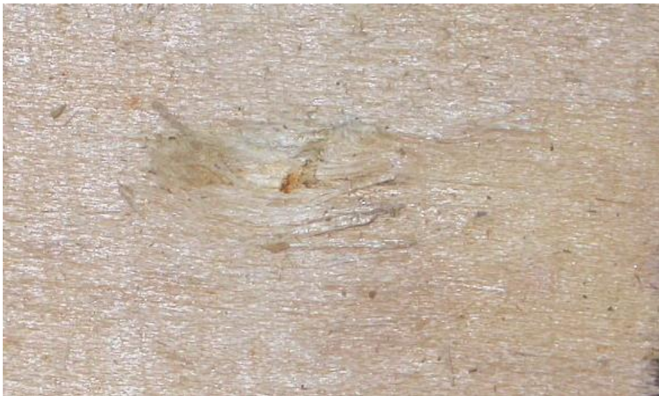
Figure 14 Sawing machine damage on a roughly-sawn sugar maple board
