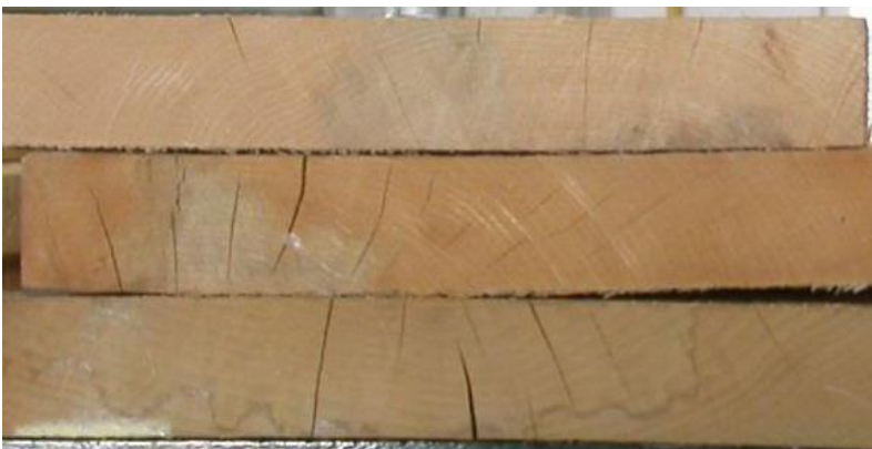
Figure 3 End checks occurred on kiln-dried boards
