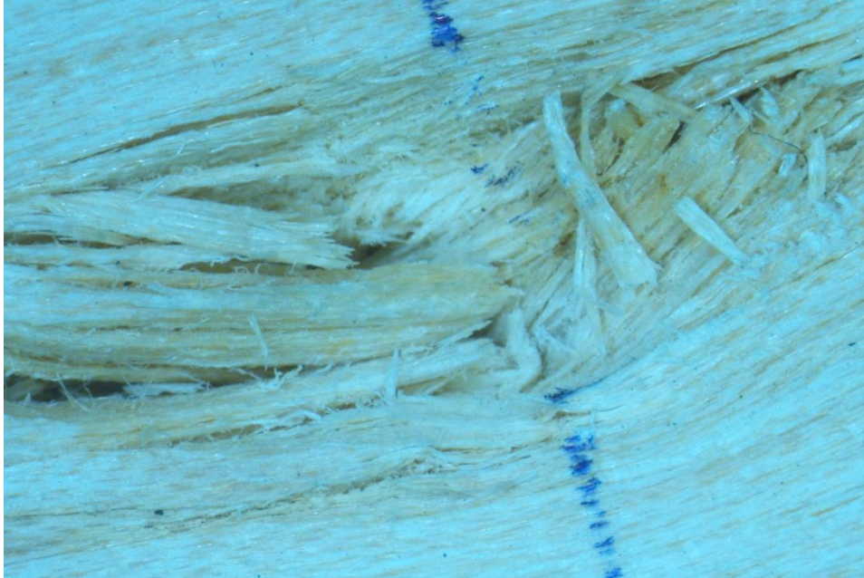
Figure 11 Magnified mechanical damage on wood surface
