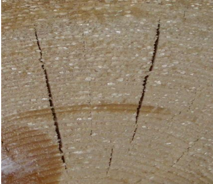
Figure 5 Internal checks formed in the middle of a thick board
